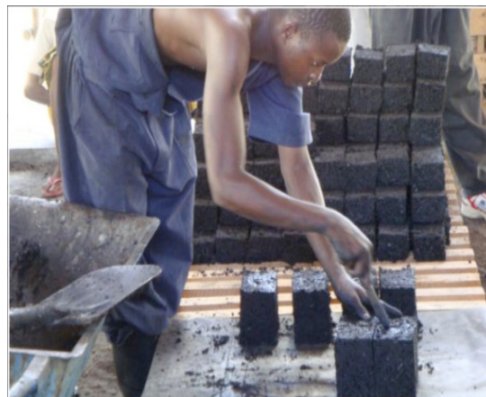
Figure 7: Charcoal substitute production (a) from bamboo (b) at MakaaZingira Sources: (a) Ethiopian Rural Energy Development and Promotion Center (b) SEED Initiative
