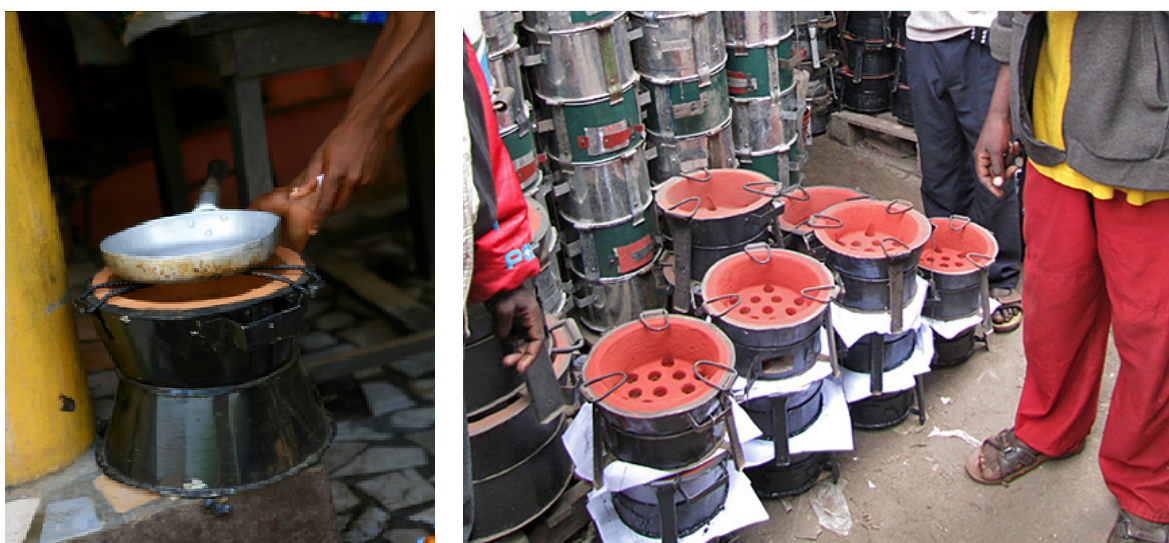
Figure 10: (a) Toyola (KCJ-type stove) in Ghana (b) KCJ stoves at the market
